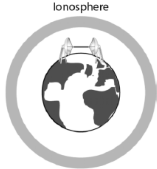
Line-of-sight propagation (above 30 MHz)
