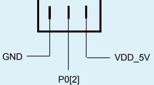
Our project was set up to output the voltage to P0[2]. So if you attach the multi-meter to the middle pin and the left pin on the Pub board, you will be able to watch the voltage decrement from 3.8 to 1.2 Volts as the LEDs count down the 256 steps.
