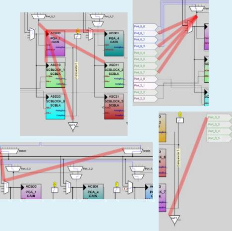
Checking "Show Allowed Connections" enables a feature that highlights all possible connections for any selected block, MUX, bus, or pin.
