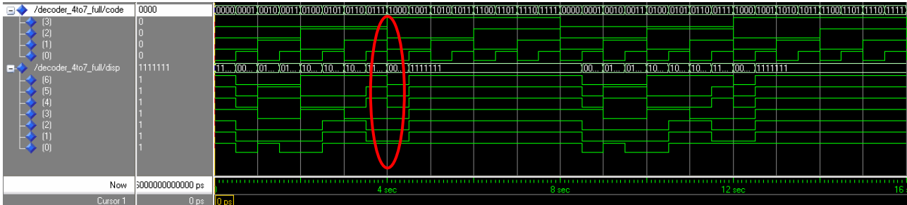
Figure 28: Timing Simulation of the Decoder
