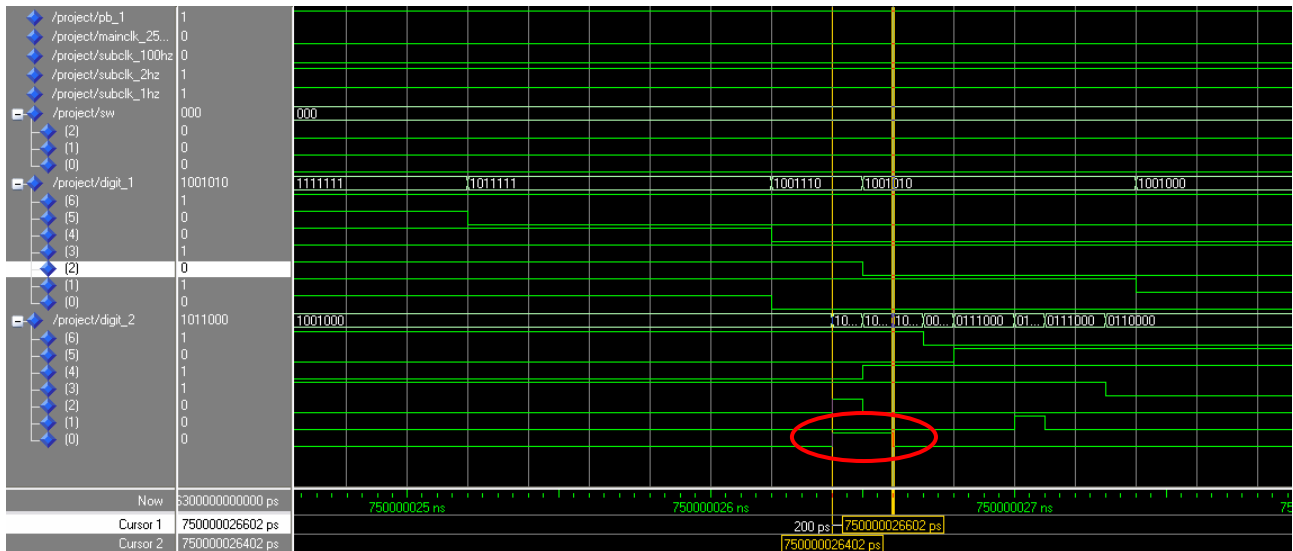
Figure 17: Further zoom on a glitch in the Timing Simulation of the simplified design
