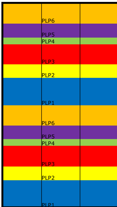
Figure 56: The matrix M_2 , showing the three rightmost columns having been moved on top of the three first columns. Each column corresponds to one RF channel (LC type D)
