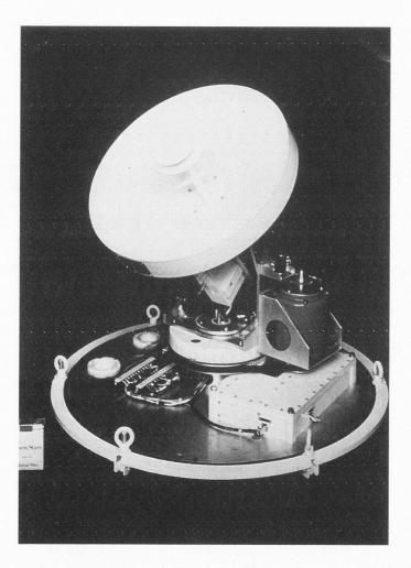
Figure 8.21 An improved SBF antenna installed on the deck for the ETS-V experiment. The antenna has a gain of 15 dBi, is 40 cm in diameter, and weighs about 40 kg including a stabilizer.
