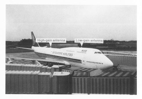
Figure 8.31 Photograph of low-gain and top-mount high-gain antennas installed on a Boeing 747.
