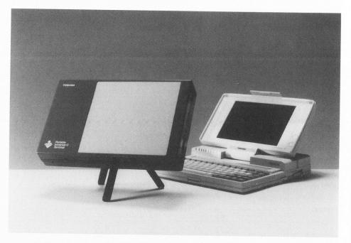
Figure 8.39 Hand-carried INMARSAT-C Earth station. A receiver with a flat antenna weighs about 4 kg and has a compact size (320 mm (W) by 210 mm (H) by 62 mm (D)). (Courtesy of Toshiba.)
