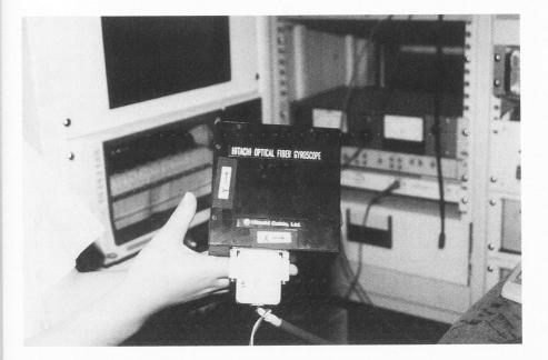
Figure 4.27 A photograph of a fiber-optic gyro.
