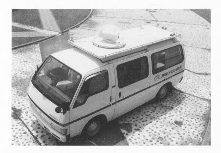
Figure 5.5 Test van for land mobile satellite propagation measurements.
