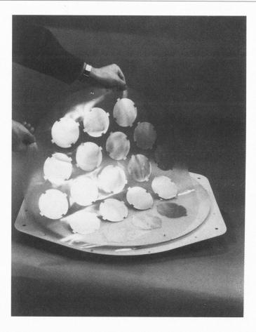
**Figure 8.36** A 19-element phased-array antenna printed on a very thin film. The *G/T* is about –13 dBK at an elevation angle of 45 degrees, and the performance was evaluated using the ETS-V satellite and an open-loop tracking method.
