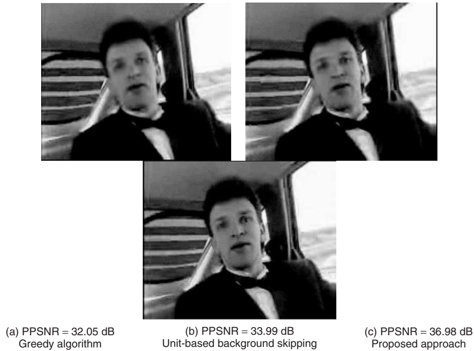
Figure 11.9 Comparison of reconstructed frames by various approaches at 48 kbps
